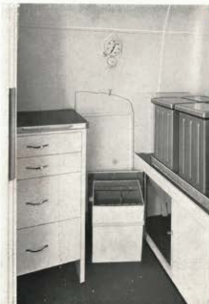
Image below: Darkroom. Right: tanks for developing and fixing baths. The drip tank for wet films is mounted on the open cabinet door. Left: cabinet with drawers for darkroom accessories.
