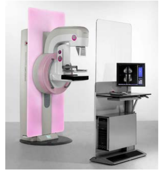
From 2012 onward, the MAMMOMAT Inspiration PRIME Edition featured a new image correction algorithm that reduced the radiation dose by up to 30 percent while maintaining the same image quality
