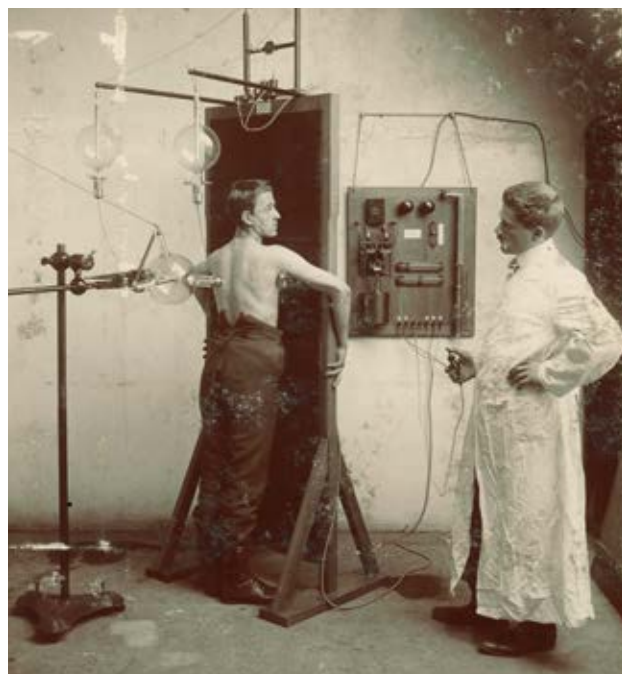
An examination using stereoscopic apparatus. The exposed high-voltage cables passed directly behind the patient, 1908
