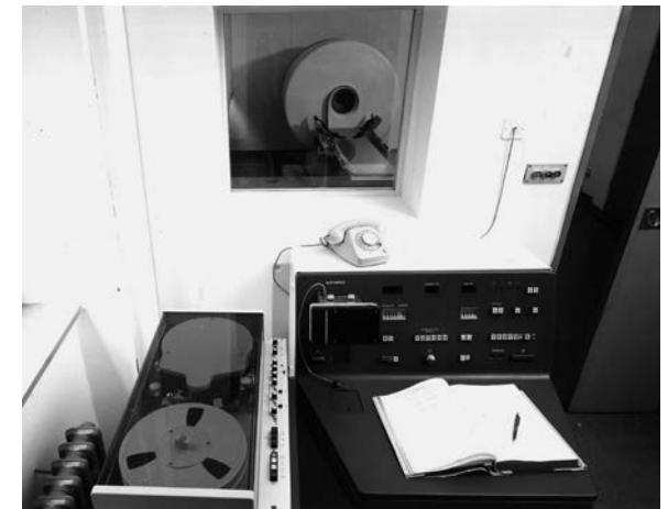
The prototype of SIRETOM with a magnetic tape storage device and a Polaroid attachment on the control desk, 1974
