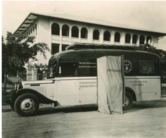
This bus is a “mobile X-ray clinic” equipped with the Orthoskop X-ray device from Siemens-Reiniger-Werke and a complete darkroom setup, among other things. It was used in the Philippines in the 1930s
