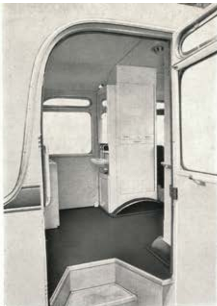
Image above: View through the rear vehicle entrance. Right: index card and filing cabinet with built-in washbasin. Left: case for the "IONTOMAT" automatic X-ray exposure timer.
