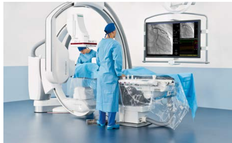
With the new X-ray tube in Artis Q and Q.zen small vessels can be visualized up to 70 percent more clearly than with previous tube technology, 2013
