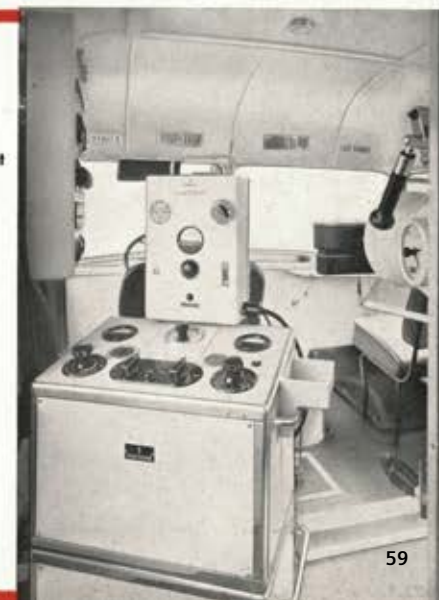
Image below: The control desk in the front of the bus with the "IONTOMAT" automatic X-ray exposure timer. Top left: control panel with fuse elements for all of the electrical installations.
