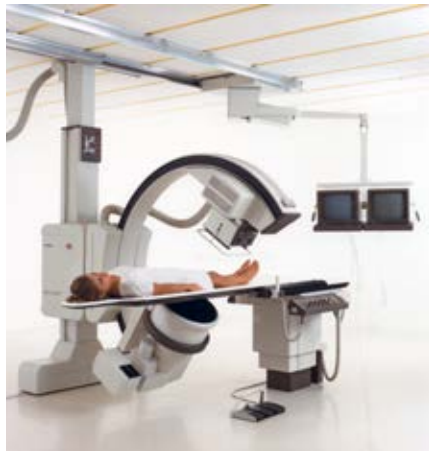
With the computer-controlled Siemens Multiskop, the C-arm takes the examination position at the push of a button, 1986
