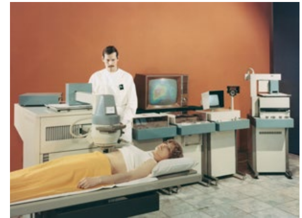
The scintigram of the SCINTIMAT 2 was displayed on a “cathode ray display device”
