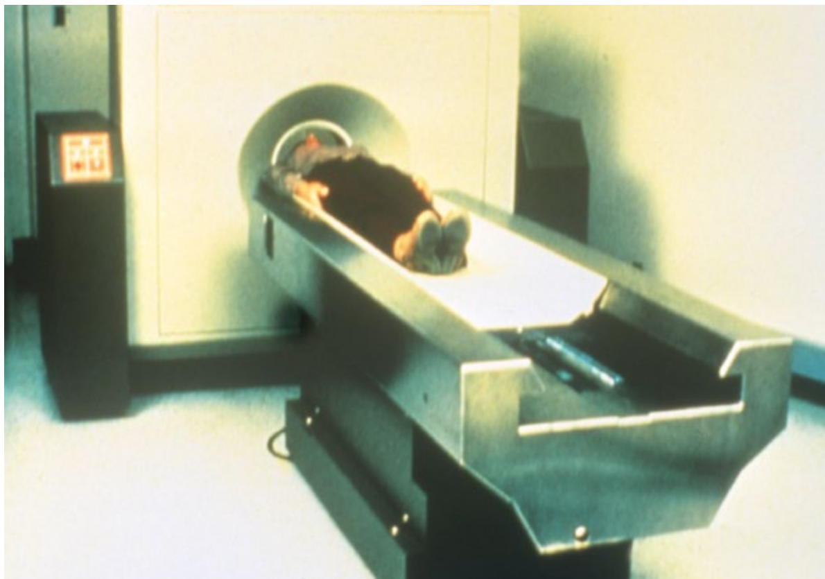
The first PET scanner with BGO elements, the NeuroECAT
