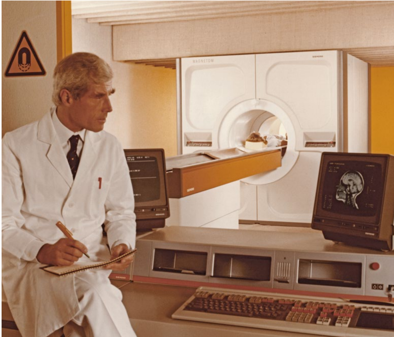
The 0.35-tesla model of the first MAGNETOM weighed around 5.3 metric tons and required at least 95 square meters of space. The 1.5-tesla model that followed slightly later weighed roughly 7.3 tons and required 140 square meters
