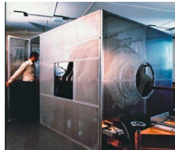
The pilot system with Faraday cage for shielding radio-frequency waves
