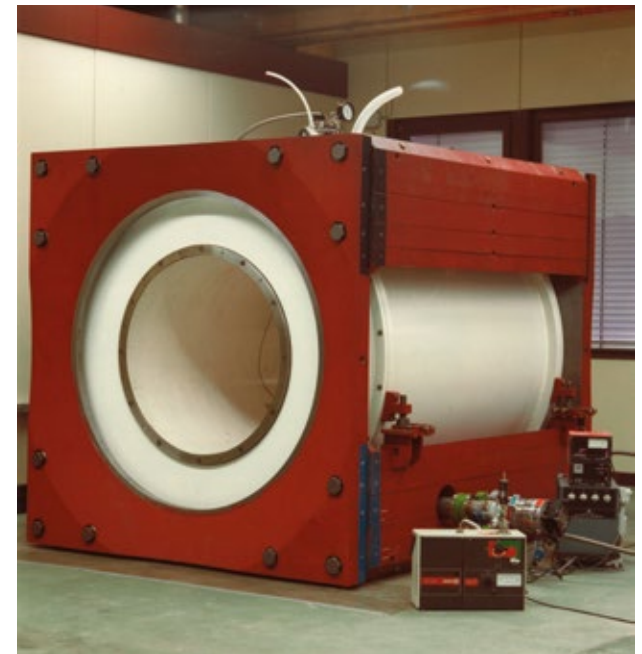
The iron shielding significantly reduced the magnet's stray field, but weighed over 30 metric tons
